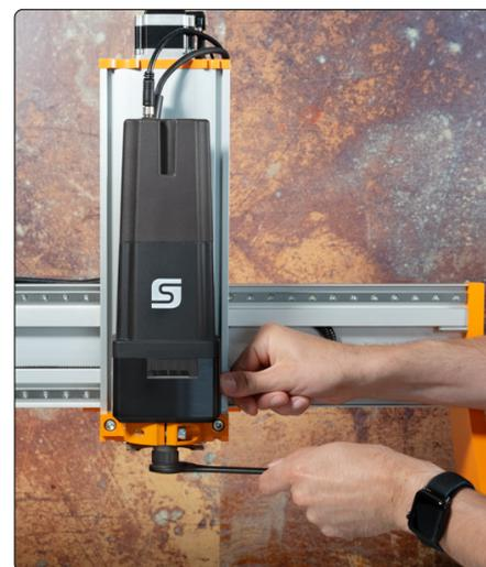
To change an OZ / 401E collet, insert the collet at an angle into the eccentric ring of the clamping nut until it audibly engages.
